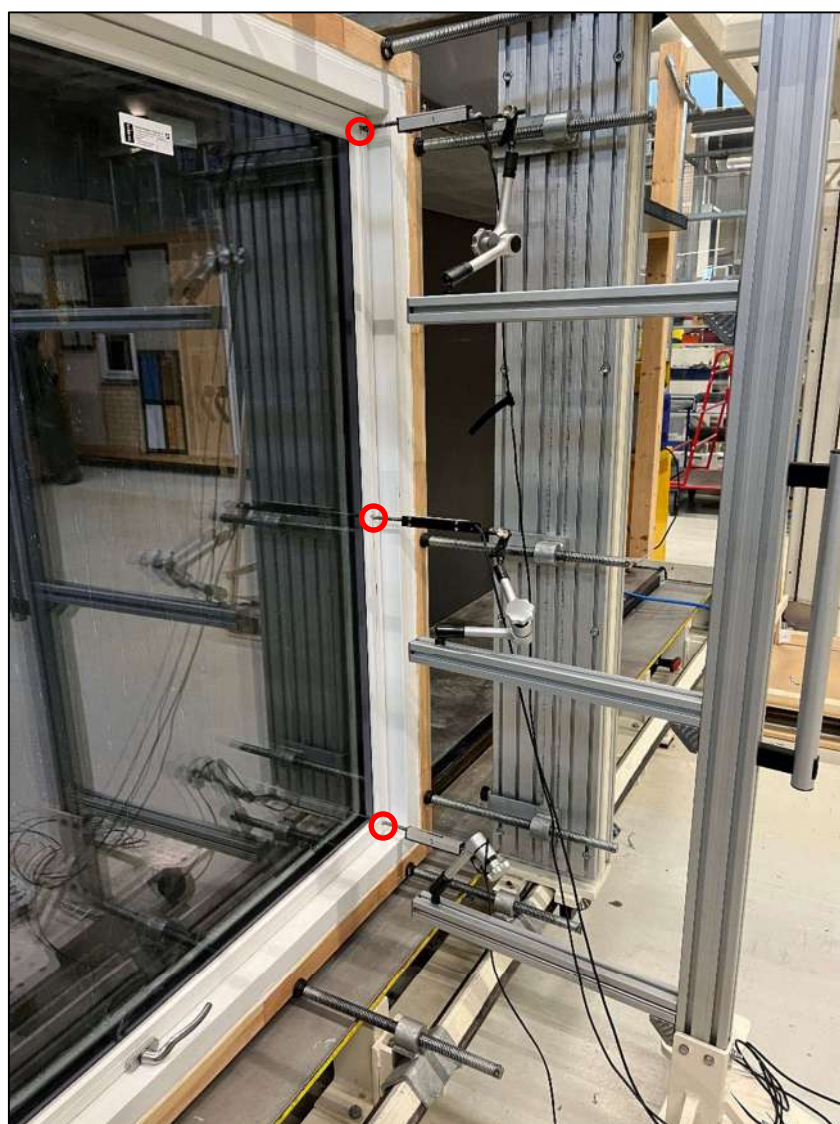
Photo 3: Test specimen during deflection test (DTI, 2022) The red circles indicate the displacement measuring points
