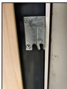
Photo 4. Hardware, both sides, broken during P3 (DTI, 2022)
